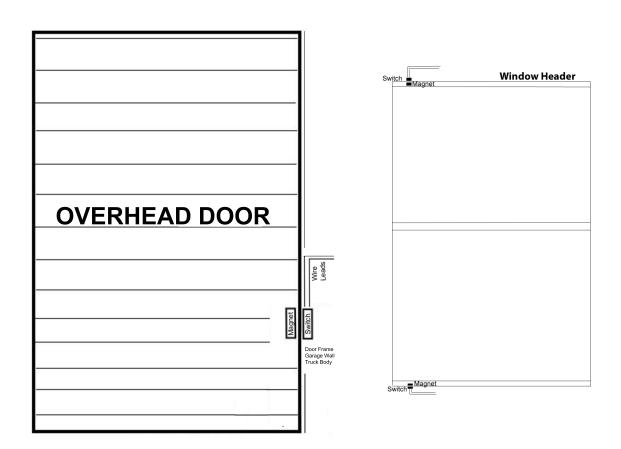
Surface mount switch on top or side of door or window frame, on garage wall or truck body Surface mount magnet parallel to the switch
